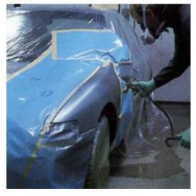
repelled (shoved away) by the paint already on the car. It also makes sure that the paint won't fall off easily, since the electrical attraction between the paint and the car is much stronger than if the paint was just sprayed on without being charged.
